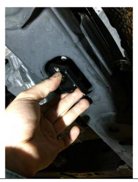
7. Insert the Internal chassis nut plate into the chassis as shown.
