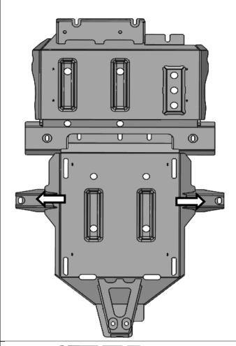
Using 2x M12x35 bolts, washers, and flange nuts, attach third panel to the side chassis braces.
